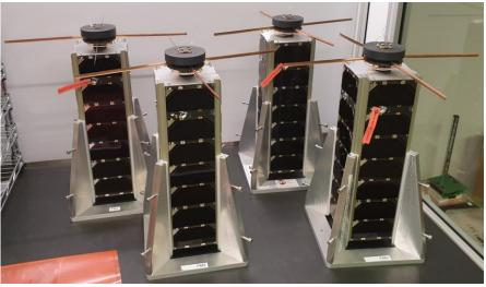
The four NetSat satellites before delivery to the launch site in a cleanroom storage
