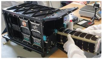
Insertion of NetSat satellites into deployer
