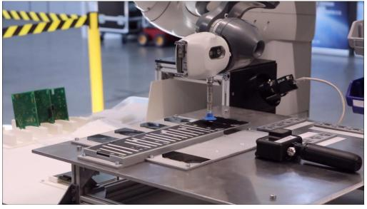
In house automated solar cell assembly using robot manipulator
